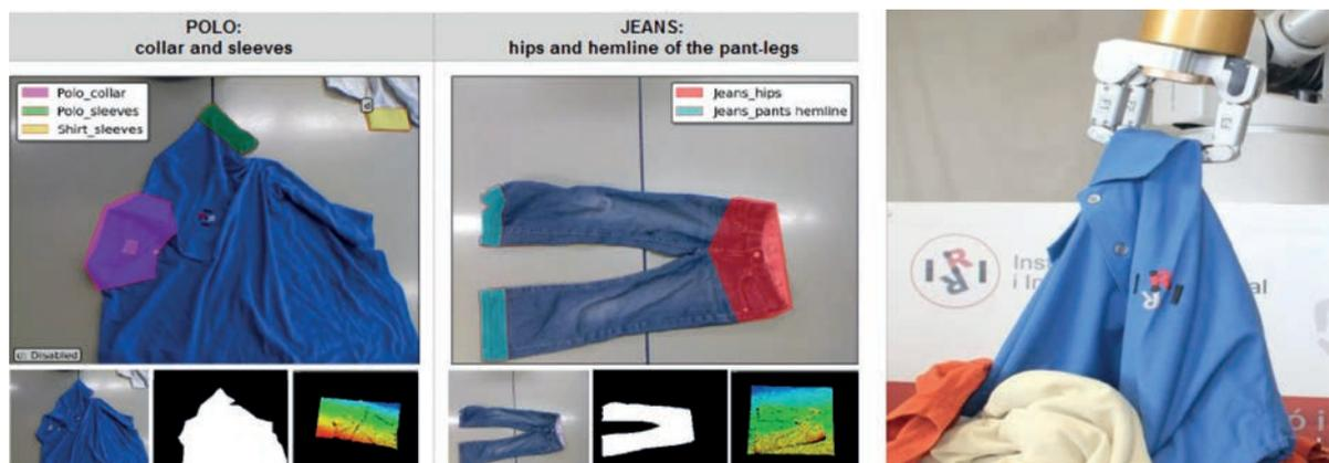
FIGURE 5. Perception and manipulation of clothes. Left: Two elements of the clothing database with the annotated parts (above), as well as the color and depth images along with the template for background subtraction (bottom). Right: The robot picks up a polo shirt by the neck to hang it.
